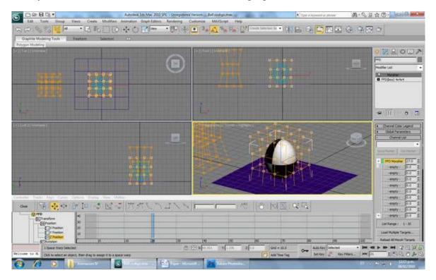
In order to squash the ball, go to Global Parameters, and make the minimum limit "-100".
