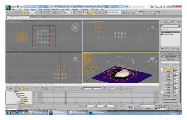
There's still one more thing. The FFD Box must move according to the floor. So let's wire it's X and Y positions. Select the FFD Box, go to Animation -> Wire Parameters, then choose Transform -> Position -> X Position.
