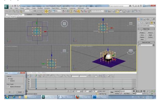
Now align the FFD Box with the ball. Select the FFD Box, then click on the align button on the Main Toolbar and select the ball.
