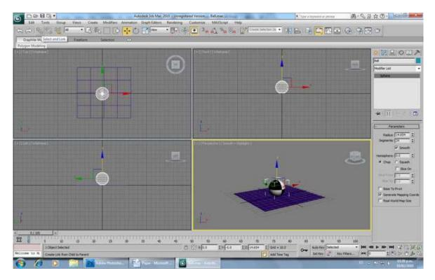
Click on the ball, keep the mouse button pressed and release it on the floor.
