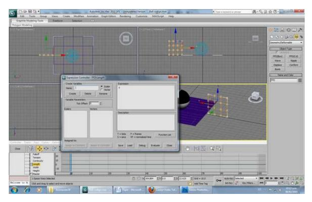
Now, you need to create the variable ballRadius. Create it, and then click on assign Controller, and go to object ball and click on radius.
