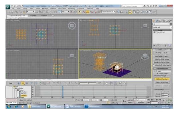
Hey, the ball doesn't change... Oh, wait a moment, we still haven't linked the ball to the FFD Box! This is easy, just click on Bond to Space Warp on the Main Toolbar, click and hold the button on the ball, and release it on the FFD Box.
