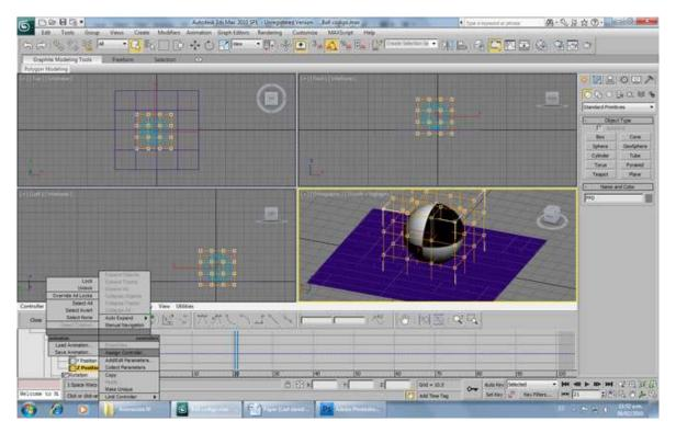
Create the variables FloorZPosition and ballRadius. Select the variable ballRadius, click on Assign to Controller, and go to ball -> Object -> Radius.
