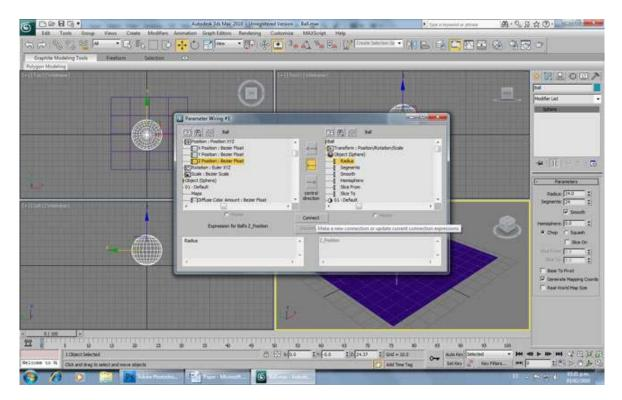
Close the window and try changing the radius of the ball in the Modify Panel of the Command Panel. You'll notice that the ball is still over the floor. This is because its position in the Z axis depends on its radius, so it'll change according to it.
