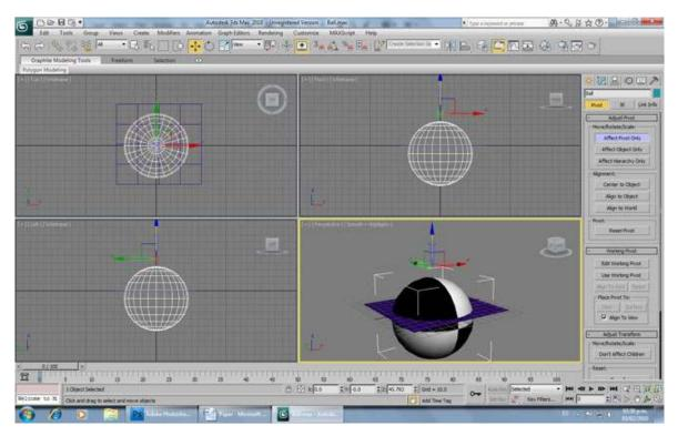
Now try moving the ball up or down. You can't. That's because the Z Position of the ball is "wired" to the radius of the ball and will always be in the center of the ball.
