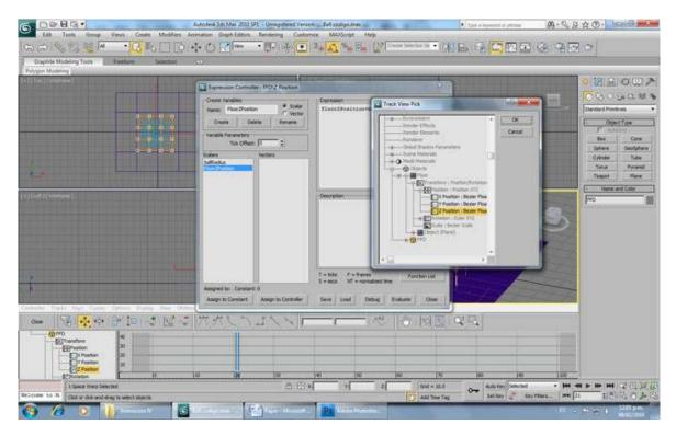
The write this code on the expression window: FloorZPosition+ballRadius. Click on evaluate and you'll see how the FFD Box follows the ball accordingly.
