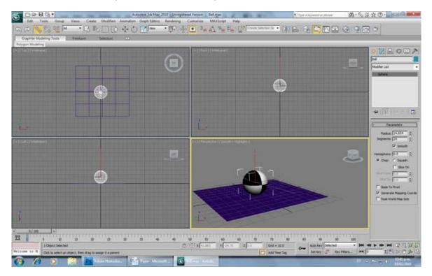
Now the floor is the ball "dad". You'll notice that when you move the floor, the ball also moves, but you still can move the ball independently. Is not "wired" like its Z Position, only "linked".
