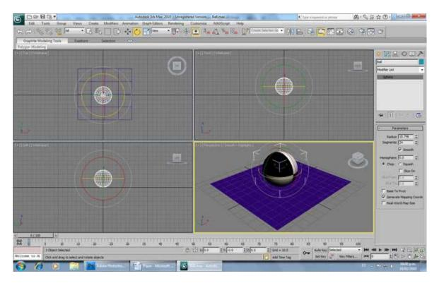
Now let's animate the ball spinning. Select the ball, go to the Time Slider menu, and click on "Auto Key". Then move the time slider to frame 50, and rotate the ball while clicking it and moving the mouse while keeping the mouse button pressed. Rotate it 90° on its X Axis and 90° on its Z Axis.
