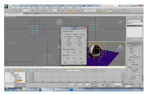
The FFD is aligned with the ball, but if you make the ball bigger, you'll notice that the FFD Box gets bigger, but doesn't goes up with the ball. Remember that the Z Position of the ball is according to the position of the floor. So you need an expression that tells the FFD Box to go up and down depending on the floor.
